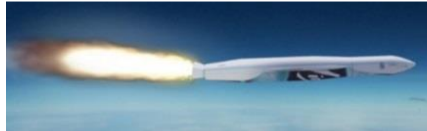
LauncherOne is a two stage RP-1 fueled 747 air launched vehicle with LOx as an oxidizer with 500 kg capabilities from Virgin Orbit.
