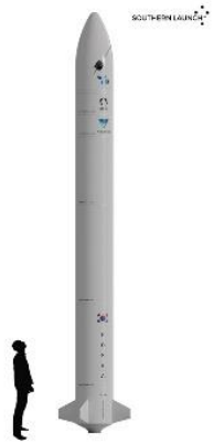
Blue Whale 1 is a two-stage ground launched vehicle with advanced engines running on LOx/LNG . ~60 kg to LEO from Perigee aerospace
